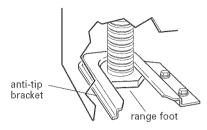
If installing the range in a mobile home, you must secure the range to the floor. Any method of securing the range is adequate as long as it conforms to the standards in the "Mobile home installation" section.
