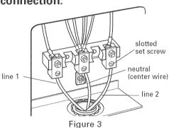
Use this method only if local codes permit connecting ground conductor to neutral supply wire.
