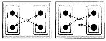
Install the parts shown below at all four surface burner locations:
