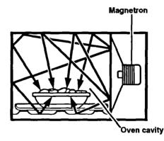
A magnetron in the microwave oven produces microwaves. The microwaves move into the oven where they contact food as it turns on the glass turntable.
