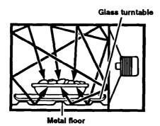
The glass turntable of your microwave oven lets microwaves pass through. Then they bounce off a metal floor, back through the glass turntable, and are absorbed by the food.
