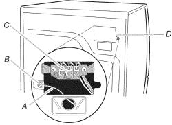
A. Neutral ground wire B. External ground conductor screw
