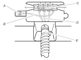
A. External ground conductor screw
