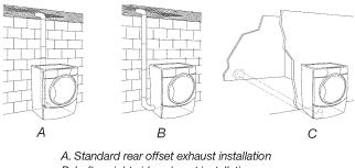
B. Left or right side exhaust installation C. Bottom exhaust installation
