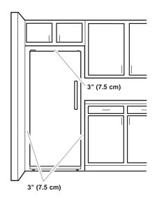
Allow at least 3 in. (7.5 cm) of air space at the top and on both sides of the freezer and 1 in. (2.5 cm) between the back of the freezer and the wall. If the freezer is to be against a wall, leave extra space on the hinge side so the door can open wider. **NOTE:** This freezer may be installed side by side with another refrigerator or freezer. Allow for a 3 in. (7.5 cm) clearance at the top and sides and a 1/4 in. (0.64 cm) clearance between the appliances.
