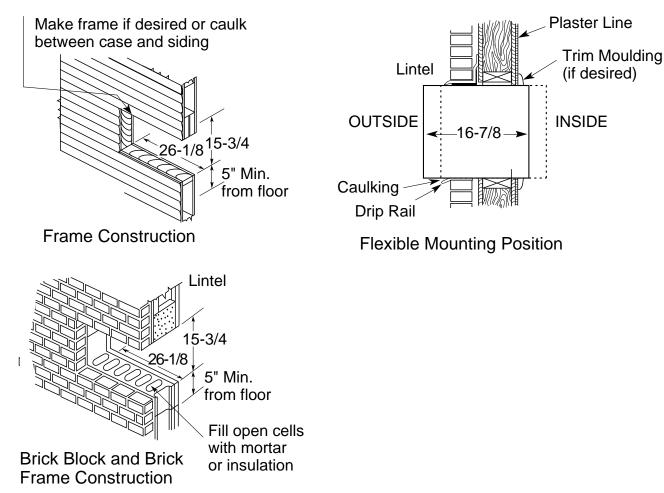
**Installation Informaion:** A finished opening of 26-1/8" x 15-3/4" clear of intrusions is required. Keep clearance of 4" from side walls. Brick veneer or frame walls should have wood studding surrounding case to provide firm anchoring with screws. Case can be fastened directly to brick or block walls with screws sunk in lead expansion shields.
