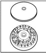
replace the burner caps. To replace the burner caps, make sure the alignment pins on the burner base are properly aligned with the cap.
