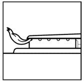
size and shape as shown. A good flame is blue in color. If the flames are uneven, you may need to clean the burners.
