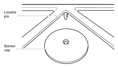
The locator pin on the grate must be positioned in the burner cap hole to hold the grate in place.
