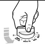
light the burners each time you turn the control knobs to LITE. Place a filled pan on
