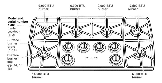
Use the left rear, center left rear, center right rear, or right front burners for simmering or for cooking smaller quantities of food requiring small cookware.
