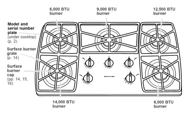
**Use the left rear, center, or right front burners** for simmering or for cooking smaller quantities of food requiring small cookware.
