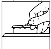
straight pin. Do not enlarge or distort the port. Do not use a wooden toothpick. If the burner needs to be adjusted, call a qualified technician for service.
