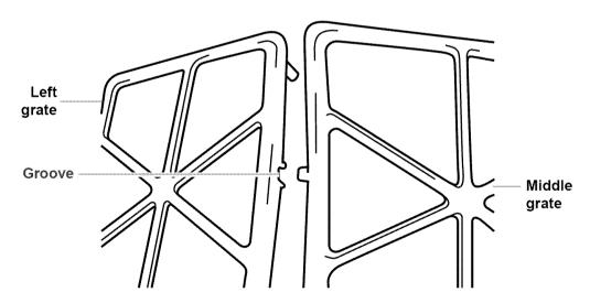
The grates located on the left and right side of the cooktop contain grooves. These grooves must always face inward toward the control knobs to hold the grates in place.
