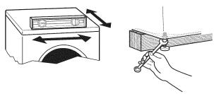
If the dryer is not level, prop up the dryer using a wood block. Use a wrench to adjust the legs up or down and check again for levelness.
