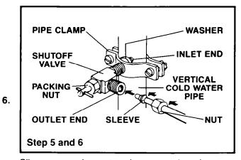
Slip compression nut and compression sleeve on copper tubing as shown in diagram. Insert end of tubing into outlet end squarely as far as it will go. Screw compression nut to outlet end with adjustable wrench. Do not overtighten. Turn ON main water supply and flush out tubing until water is clear. Turn
