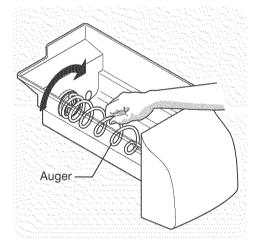
**IMPORTANT:** When removing or replacing the ice bin, do not rotate the auger in the ice bin. If the auger is accidentally turned, you must realign the auger by turning it in 90° turns until the ice bin fits into place with the drive mechanism.
