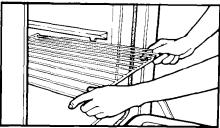
**1.** Position the rack(s) properly before turning on the oven. To front and pull out.
