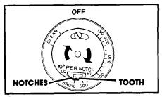
**4.** To raise the temperature, move the tooth a notch closer to HI. Each notch equals about 10°F (5°C).
