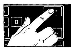
5. Touch START. The oven will start the Self-Cleaning cycle automatically at the time you have set. The Lower Oven LOCKED Signal Light will come on when the oven temperature exceeds normal baking temperatures. The Lock Lever must not be moved and the door can't be opened when this light is on.
