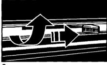
Lift the panel between the upper and lower oven doors. Move the Lock Lever all the way to the right.
