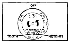
**3. To lower the temperature,** move the tooth a notch closer to LO. Each notch equals about 10°F (5°C).
