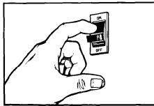
WARNING: To avoid possible shock hazard, turn off the electric power at the main power supply.
