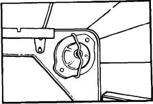
4. Replace the bulb cover and snap the wire holder in place. Turn the power back on at the main power supply.
