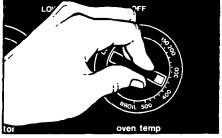
**3.** Set the Oven Temperature Control on the baking temperature you want The Lower Oven HEATING Signal Light will come on. The oven is preheated when the Lower Oven HEATING Signal Light first goes off.
