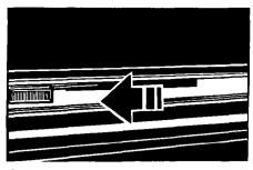
6. After the Self-Cleaning cycle is completed, the Lower Oven LOCKED Signal Light goes off. Move the Lock Lever back to the left. Do not force it. Wait until it will move easily.
