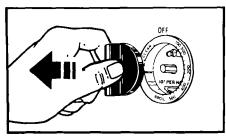
**1.** Pull the Oven Temperature Control Knob straight off.
