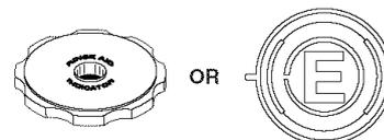
Or you can remove the Fill Indicator cap. If an “E” is visible, the dispenser is empty.
