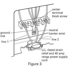
Use this method only if local codes permit connecting cabinet-ground conductor to neutral wire of power supply cord.
