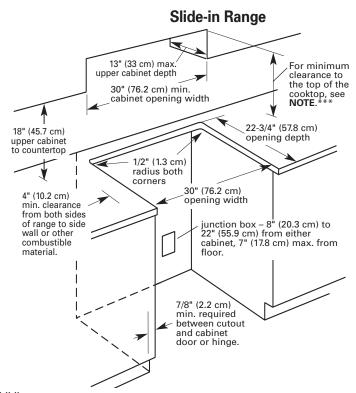
\*\*\* NOTE: 24" (61 cm) min. when bottom of wood or metal cabinet is protected by not less than 1/4" (0.64 cm) flame retardant millboard covered with not less than No. 28 MSG sheet steel, 0.015" (0.4 mm) stainless steel, 0.024" (0.6 mm) aluminum or 0.020" (0.5 mm) copper.
