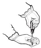
**6** ■ Use the anti-tip bracket template to install the anti-tip bracket.
