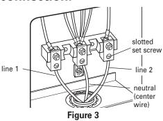
Use this method only if local codes permit connecting ground conductor to neutral supply wire.
