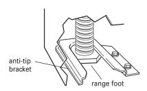
**12** Making sure the anti-tip bracket is installed:
