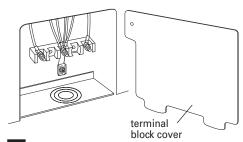
Remove the terminal block cover located on the back of range.
