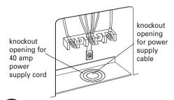
Depending on your electrical supply, make the four-wire or three-wire connection to the range following the "Power supply cord method" or "Direct wire method" instructions for copper wire or aluminum wire depending on the connection needed.
