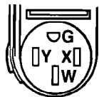
4-wire wall receptacle (14-50R) Figure 1
