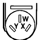
3-wire wall receptacle (10-50R) Figure 2
