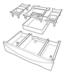
**3** To clean the drawer opening, use a small, non-metal brush to clean the recess. Remove all residue from the upper and lower parts of the recess.
