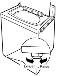
If the washer is not level, adjust the front leveling legs. Turn clockwise to raise, counterclockwise to lower.
