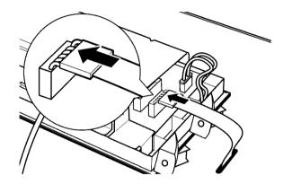
Place the ribbon and the wire from the rear cover under the strain relief on the new backsplash.
