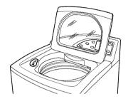
**Wash Basket:** Leave the lid open after washing to allow moisture to evaporate. If you want to clean the basket, use a clean soft cloth dampened with liquid detergent; then rinse. (Do not use harsh or gritty cleaners.)
