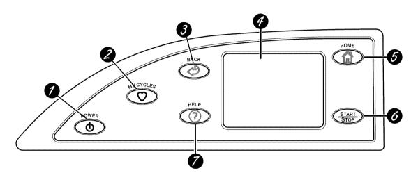
Features of the washer control panel 1 **POWER.** Press to "wake up" the display. If the display is active, press to put the washer into standby mode. If there is no screen activity for 5 minutes the display will turn off. You may also press the Touch Screen or any button to "wake up" the display.
