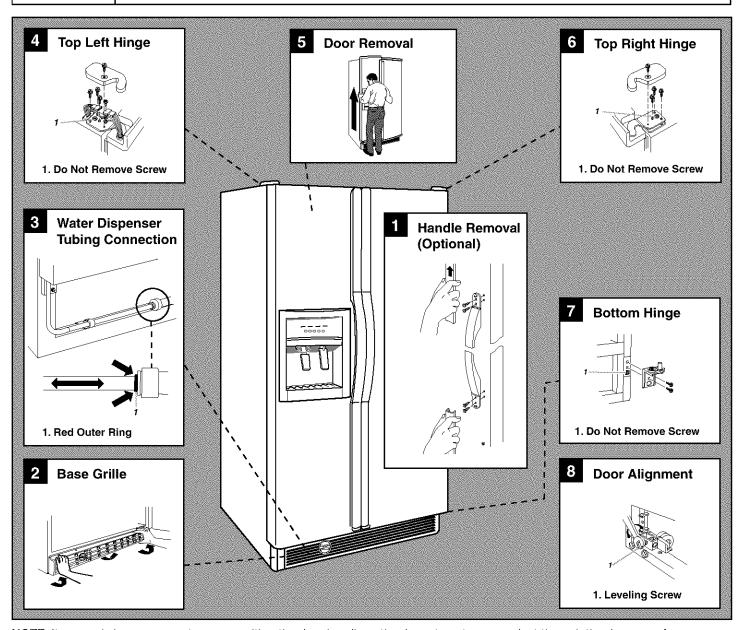
**NOTE:** It may only be necessary to remove either the door handle or the doors to get your product through the doorway of your residence. Measure the door opening to determine whether to remove the refrigerator handles or the doors.
