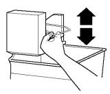
Install the interior water filter cartridge (on some models). The interior water filter mounting bracket is located in the upper corner of the fresh food compartment of the refrigerator.
