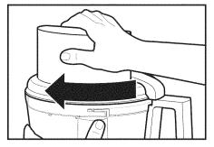
If using a disc, remove it before removing the bowl. Holding the disc by the 2 finger grips, lift it straight up. Remove the adapter when using the Shredding Disc.
