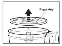
**5.** If using the mini-bowl, grasp and remove the bowl using the finger grips located along the top edge of the bowl.
