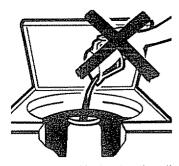
Do not pour anything into the agitator if the agitator cap or dispenser is removed.
