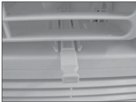
Figure 3 (VENT & EXHAUST OPEN)
