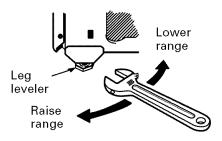
D Use an open-end or adjustable wrench to adjust the leveling legs until the range is level.
