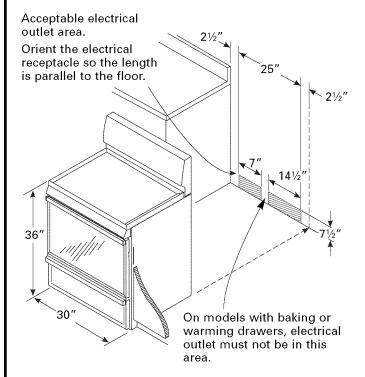
**NOTE:** Use a 4' power cord to prevent interference with the storage drawer. Power cords 4½ to 6' long may have to be dressed to allow for proper drawer closing.
