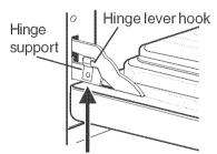
Lock engaged for door removal Figure 1
