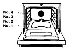
Your oven has three racks. Two racks are straight and the third is offset (raised). The shape of the offset rack helps you space racks better.
