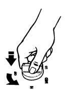
2. After the burner lights, turn the control knob to the desired setting.
