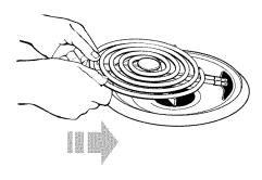
**4.** When the terminal is pushed into the receptacle as far as it will go, push down the edge of the coil element opposite the receptacle.
