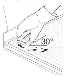
If soils remain, carefully scrape soils with a metal razor blade scraper, holding scraper at a 30 degree angle to the surface. Remove loosened soils with cooktop cleaning cream and buff surface clean.
