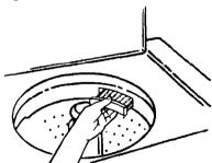
To remove it for cleaning, twist it clockwise and pull straight out. Instructions for cleaning are printed on the bottom of the filter.
