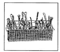
Load knives and fork with handles up. Be sure items do not protrude through the holes in the basket and stop the rotation of the spray arm.
