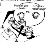
the regulator. Natural gas spuds are brass and LP gas spuds are red or silver. (Mount the spuds that you removed from the inlet tubes back in the holder.) To prevent leakage, make sure spuds are securely screwed into gas inlet tubes.
