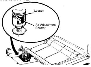
The shutter for the bottom (oven) burner is near the back wall behind the storage drawer or the kick panel (depending on the model). Remove the drawer or panel. See the Care and Cleaning section in this guide.
