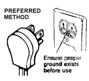
wall receptacle to minimize the possibility of electric shock hazard from this appliance. The customer should have the wall receptacle and circuit checked by a
