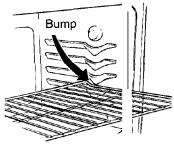
When placing cookware on a shelf, pull the shelf out to the bump on the shelf support. Place the cookware on the shelf, then slide the shelf back into the oven. This will eliminate reaching into the hot oven.
