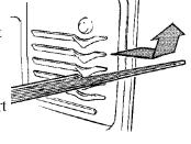
shelf) facing up and toward the rear of the oven. Tilt up the front and push the shelf toward the back of the-oven until it goes past the bump on the shelf support. Then lower the front of the shelf and push it all the way back.
