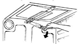
To convert to LP gas, use a 1/2" wrench to turn the upper burner orifice spud clockwise. Tighten spud only until it is snug with the base. To prevent damage, do not overtighten spud.
