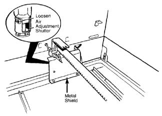
Remove the metal shield at the rear of the cavity. The air adjustment shutter is behind this shield. To adjust the flow of air to the burner, loosen the Phillips-head screw and rotate the shutter to allow more or less air into the burner tube.
