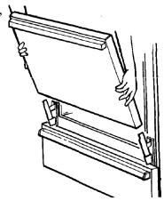
To **replace the door**, make sure the hinges are in the special stop position. Position the slots in the bottom of the door squarely over the hinges. Then lower the door slowly and evenly over both hinges at the same time. If hinges snap back against the oven frame, pull them back out.
