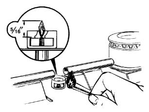
**NOTE:** Do not leave standing pilot lit in a newly constructed or remodeled home or apartment that will be unoccupied for more than a month. Each pilot flame was adjusted at the factory to be approximately 5/16" tall. A tinge of yellow appearing at the upper tip is normal. If you find pilot adjustment is necessary, follow instructions at right.
