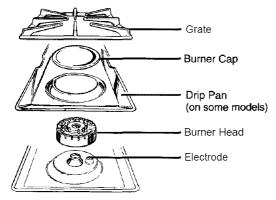
Turn all controls OFF before removing the burner parts and drip pans (if so equipped).
