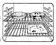
Do not put aluminum foil on the oven bottom.
