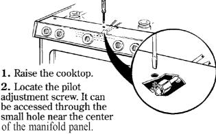
3. To adjust, use a blade-type screwdriver with a shaft diameter of less than 3/16". Turn pilot adjustment screw until pilot is 5/16" high. Do not reduce the flame to less than 5/16" or pilot outage may occur. A pilot flame burning higher than recommended may generate soot (carbon black) on the bottom of your cooktop.
