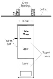
**Note:** The cross framing must be spaced 8-3/4" on the side from centerline to centerline in order to accept the hood mounting screws.
