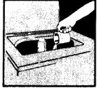
4. Run the washer through a complete cycle with one cup of detergent to clean out the antifreeze.
