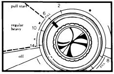
HIGH WATER LEVEL. The washer will automatically fill to its highest level, (about 20.5 gals./77.6 L), when the Control Knob points to a FILL area.
