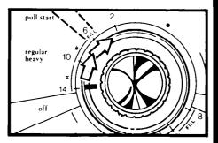
**LOWER WATER LEVELS.** Setting the washer to fill with less water also sets it for a shorter wash time.
