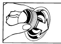
A. Push in the Control Knob and turn it to the right. It must be pushed in and turned only clockwise.
