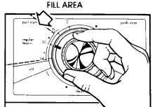
**B.** Stop on a number in the cycle you want. The numbers are minutes of wash time. The drawing shows 10 minutes of agitation in the REGULAR HEAVY Cycle. **NOTE:** The washer will fill only when the knob points to a FILL area.
