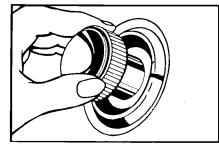
C. Start the washer by pulling out the Control Knob. After filling, the washer will agitate for the selected number of minutes.
