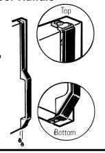
**5.4.3** Remove the screw from the right top edge of the door and insert it into the handle screw hole on the left side.
