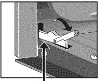
Lock engaged for door removal
