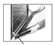
HINGE SLOT-Door removed from the appliance
