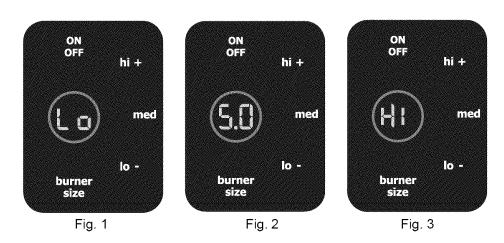
The **hi+** and **lo-** keys provide incremental adjustments for more precise control when changing settings between the lower heat levels (Lo to 3.0 power levels). Higher heat level setting changes (between 3.0 to HI) will change much faster.
