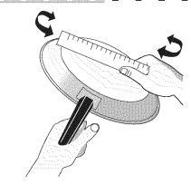
Cookware should have flat bottoms that make good contact with the entire surface heating element. Check for flatness by rotating a ruler across the bottom of cookware. Be sure to follow the recommendations for using cookware that is shown in the illustrations at right.
