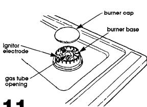
Put burner caps on each burner base. Place burner grates over burner bases and caps.
