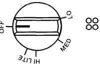
12 Check the operation of the cooktop burners. Push in and turn each control knob to "LITE" position. The flame should light within 4 seconds. Do Not leave the knob in the "LITE" position after burner lights.
