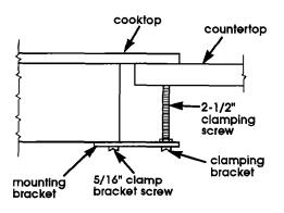
Rotate mounting brackets away from burner box. Tighten the mounting brackets to the burner box. Insert the 2-1/2" clamping screws into the mounting brackets. Use a screwdriver to tighten screws against the underside of countertop.
