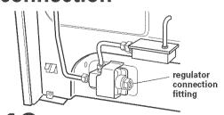
Assemble the flexible connector to the gas supply pipe to the pressure regulator connection fitting, using the adapter fittings provided with the flexible connector. Use pipe-joint compound made for use with L.P. gas to seal all pipe thread connections.
