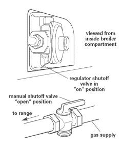
Check that range regulator shutoff valve is in the "on" position. Open the manual shutoff valve in the gas supply line.
