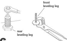
Remove cardboard shipping base from under range. Open broiler door. Use a 3/8" drive ratchet to lower rear leveling legs one-half turn. Use slip-joint pliers to lower front leveling legs one-half turn.
