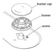
Remove burner grates, burner caps, burners and screws. Lift cooktop. Note: There is no cooktop support rod.
