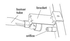
**c.** Lift front of bracket and push tube and bracket assembly back off orifice.
