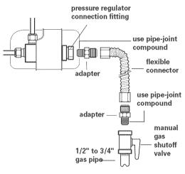
A 1/2" male pipe thread is needed for connection to pressure regulator female pipe threads.
