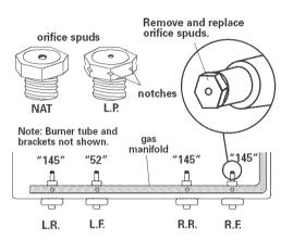
d. Locate Natural gas orifice spuds for top burners in literature package included with the range. Three Natural gas spuds are stamped "145" and one "52". Remove Natural gas orifice spuds using a 3/8" combination wrench. Install Natural gas orifice spuds in locations shown to replace the L.P. gas orifice spuds. Note: Depending on model, the range cooktop may be equipped with 4 standard burners or 3 standard burners and 1 power burner. Spud size/location remain the same.
