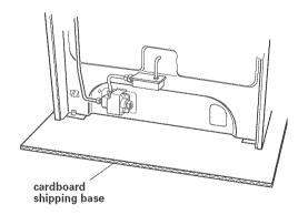
• Keep cardboard shipping base under range to prevent damage to floor covering.
