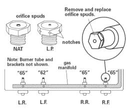
d. Locate L.P. gas orifice spuds for top burners in literature package included with the range. Three L.P. gas spuds are stamped "65" and one "62". Remove Natural gas orifice spuds using a 3/8" combination wrench. Install L.P. gas orifice spuds in locations shown to replace the Natural gas orifice spuds. Note: Depending on model, the range cooktop may be equipped with 4 standard burners or 3 standard burners and 1 power burner. Spud size/location remain the same.
