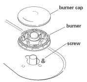
Remove burner grates, burner caps, burners and screws. Lift cooktop. Note: There is no cooktop support rod.
