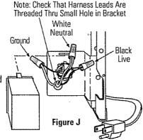
the stripped ends. Using UL Listed wire nuts of appropriate size, connect incoming white to white, black to black, and incoming ground to green wire. Replace the junction box cover. Check that wires are not pinched under cover.
