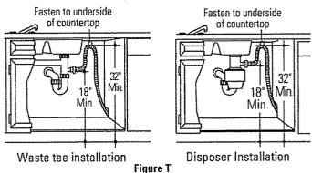
**Note:** BE SURE TO REMOVE DRAIN PLUG FROM DISPOSER BEFORE ATTACHING DRAIN LINE. DISHWASHER WILL NOT DRAIN IF PLUG IS LEFT IN PLACE.
