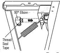
Do not bend the dishwasher frame when installing the 90° elbow fitting to the water valve as this could cause the door spring to come in contact with the fill hose.
