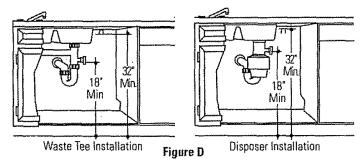
Install waste tee or disposer and air gap according to manufacturer's instructions.
