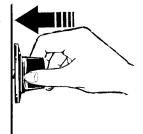
When one burner is turned to LITE, *all* the burners spark. Do not attempt to disassemble or clean around any burner while another burner is on. An electric shock may result, which could cause you to knock over hot cookware.
