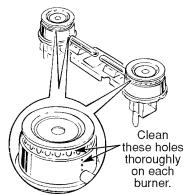
You should clean the surface burners routinely, especially after bad spillovers, which could clog these holes. Wipe off surface burners. If heavy spillover occurs, remove the surface burners from the range. Burners lift out for cleaning. Lift up the cooktop and then lift out the surface burners.
