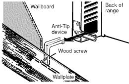
**5.** Slide the range against the wall, and check for proper installation by grasping the front edge of the cooktop and carefully attempting to tilt the range forward.
