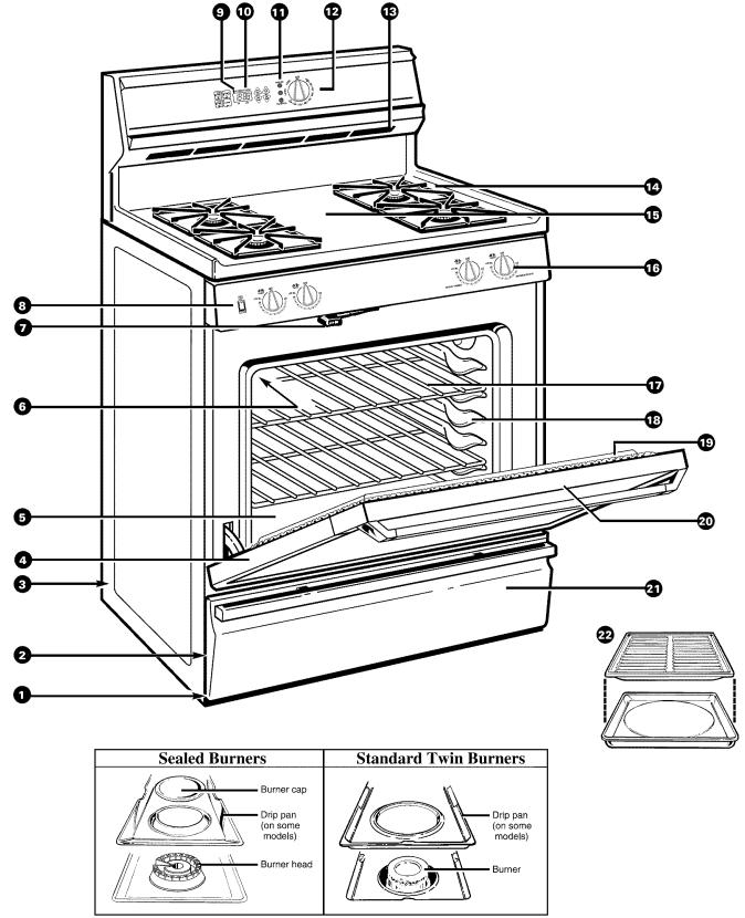
Your range is equipped with one of the two types of surface burners shown above.
