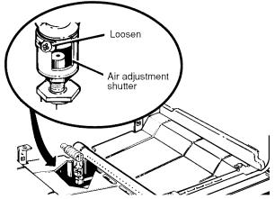
The shutter for the bottom (oven) burner is near the back wall behind the kick panel. Remove the panel. See the Care and Cleaning section in this guide.
