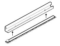
**B** Install the top mounting rail with 3 type A screws from the outside of the case.
