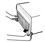
**C** Lift the top of the grille up and off to release from the tabs.
