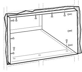
**C** Place the case in the wall opening and secure with 12 1" long #10 wood screws.
