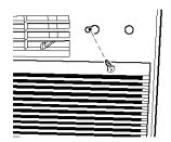
On some models, remove the knobs, filter and screw behind the filter bottom.
