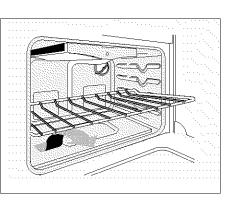
**To remove an oven rack**, pull the rack forward until it stops. Lift up front of rack and slide out. **To replace an oven rack**, fit the rack onto the guides on the oven walls. Tilt the front of the rack upward and slide the rack back into place.
