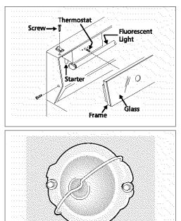
**CAUTION** Be sure the oven is unplugged and all parts are COOL before replacing the oven light. Wear a leather-faced glove for protection against possible broken glass.
