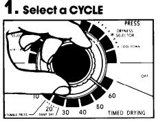
Turn the Control Knob either way to point to the cycle and setting you want. See page 6 for information on the cycles.
