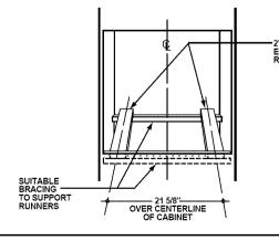
If the cabinet does not have a solid bottom, then two braces and runners must be installed to support the weight of the oven. For double ovens the runners and braces must support 275 pounds.
