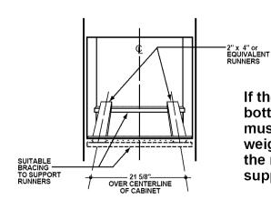
If the cabinet does not have a solid bottom, then two braces or runners must be installed to support the weight of the oven. For single ovens the runners and braces must support 150 pounds.
