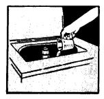
Run the washer through a complete cycle with one cup of detergent to clean out the antifreeze.
