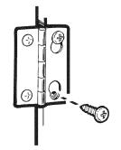
Remove the remaining screws from the side of the opening from which the door was removed. With these screws, secure each hinge at the bottom. Tighten the two top screws of each hinge. Reinsert the plastic plugs on the side from which the door was removed.
