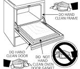
To clean oven door, wash with hot, soapy water and a clean cloth. DO NOT immerse the door in water.
