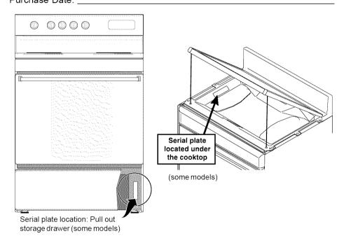
The product serial plate will provide you both the model number and serial number for your range. You can find the serial plate on your range at one of the locations illustrated above.
