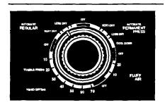
Select a cycle by turning the Cycle Control Knob either way. Stop when the indicator on the knob's outer ring points to the cycle and setting you want. See pages 6-8 for further cycle information.
