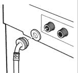
outlet of the water value. Tighten by hand; then tighten another 2/3 turn with pliers. Do not crossthread or over-tighten these connections.
