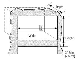
On 27" (68.6 cm) models, allow 1" (2.5 cm) at the top,  $^{11}/_{16}$ " (1.75 cm) on the sides and 1%" (3.5 cm) at the bottom for overlap of the Trim Frame over the edges of the cutout.
