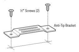
Install the anti-tip bracket onto the cutout floor using two ½" screws.
