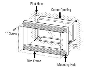
**D** Attach the trim frame by using four screws.
