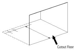
**B** Remove the template and drill two holes for the anti-tip bracket.
