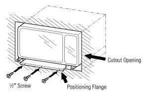
F Drill pilot holes through the positioning flange and then install three ½" screws at the front of the bottom duct as shown.
