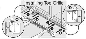
4 Close the doors. Fasten right and left side clips into groove of bottom hinge.
