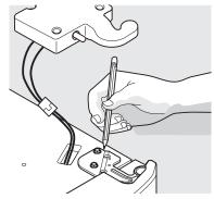
2 Remove the two screws from the top hinge. Lift the door off of the bottom hinge and set it aside.
