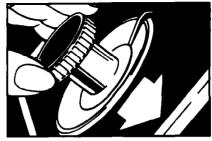
**D.** To stop the washer at any time push in the Control Knob. To restart the washer, pull out the Control Knob. STARTING YOUR WASHER
