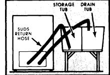
The SUDS-MISER® System stores a portion of the wash water. If you have a storage tub big enough to hold 25 gallons (95 liters) of water, you can have a qualified installer convert your washer to save more of the water.
