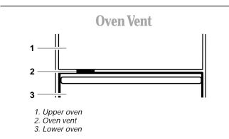
The oven vent should not be blocked or covered since it allows the release of hot air and moisture from the oven. Doing so will cause poor air circulation, affecting cooking and cleaning results. Never set plastics, paper or other items that could melt or burn near the oven vent.
