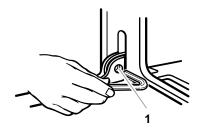
1. Insert small end of pin here
