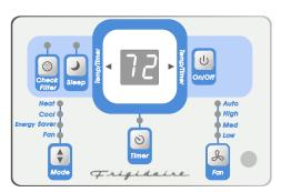
**NOTE:** Tap or hold either up( $\blacktriangleleft$ ) or down( $\blacktriangleright$ ) button until the desired temperature is seen on the display. This temperature will be automatically maintained anywhere between 60°F(15°C) and 90°F(32°C). If you want the display to read the actual room temperature. See "To Operate on Fan Only" section on Page 7.
