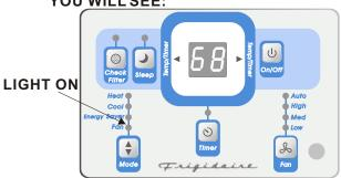
**NOTE:** Use this function only when cooling is not desired, such as for roomair circulation or to exhaust stale air. (Remember to open vent during this function, but keep it closed during cooling for maximum cooling efficiency.) You can choose any fan speed you prefer.
