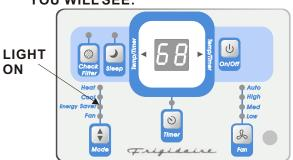
NOTE: In this mode, the fan will continue to run for 3 minutes after the compressor shuts off. The fan then cycles on for 2 minutes at 10 minute intervals until the room temperature is above the set temperature, at which time the compressor turns back on and cooling starts.
