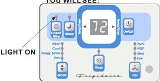
NOTE: This feature is a reminder to clean the Air Filter (See Care and Cleaning) for more efficient operation. The LED (light) will illuminate after 250 hours of operation. To reset after cleaning the filter, press the "Check Filter "button and the light will go off.
