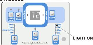
NOTE: Fan starts at High Speed and adjusts to a slower speed as the room temperature dictates. For example if the room does not get too warm, it will stay at the slowest speed. If the room temperature rises quickly, such as a door being opened, it will automatically go to the highest speed. The fan speeds will re-adjust back to the slowest speed as the room returns to the original set temperature. Press the fan button to adjust the fan speed manually.
