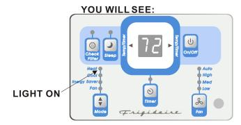
**NOTE:** This feature can be used with any combination of FAN Speeds, Timer, or Sleep Modes. When in the Heat Mode, the fan will run continuously while heat is needed. The temperature will automatically be maintained anywhere between  $60^{\circ}F(15^{\circ}C)$  and  $90^{\circ}F(32^{\circ}C)$ . When the room set temperature is satisfied, the fan will cycle off and on to circulate and sample the room air.
