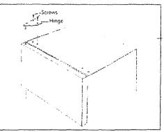
**13.** Assemble upper hinge (and shim on some models) to top of cabinet and door Use opposite set of holes. Do not completely tighten screws
