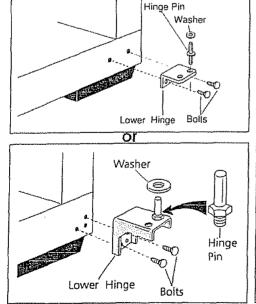
4. Remove hinge pin, hinge, and the two 5. Carefully remove the hole plugs from bolts attaching the lower hinge. Save the the hinge holes in the center mullion and hinge, hinge pin, washer (some top of cabinet and reinstall in the opposite models) and bolts for reassembly later. set of holes
