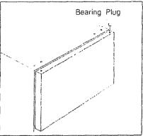
**12.** Remove plug from upper bearing of door and reinstall on opposite side
