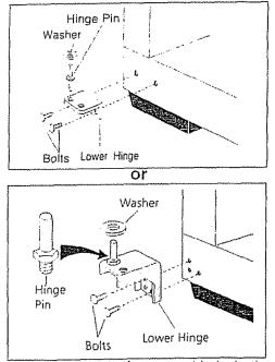
9. Using a putty knife. remove black plastic plug (in some models) from front of base, and reinstall in opposite set of lower hinge holes Assemble lower hinge to cabinet Install hinge pin in opposite hinge hole from which it was removed Install the washer (some models) on the lower hinge pin and insert hinge bolts. but do not tighten Hinges will have to remain loose against cabinet to align door
