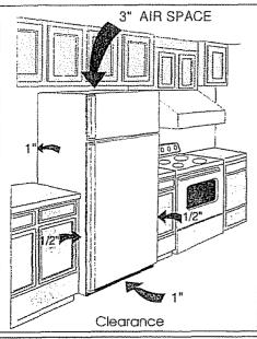
Proper air circulation and leveling will ensure efficient operation.
