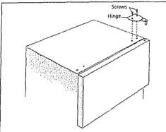
(some models). With the freezer door it to be lifted off the center hinge closed, remove the two screws attaching upper hinge to cabinet Lift the hinge up and off On some models, remove the shim also. Be sure to save screws, (shim), and hinge for reassembly later.
