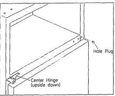
**10.** Turn center hinge upside down and secure to cabinet as shown, using the screws which are in the new holes Install refrigerator door on lower hinge pin Align door with edge of cabinet Hold the door on front of cabinet
