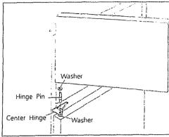
**11.** Place original washer (some models) over hole in refrigerator door and line up hole in center hinge Insert hinge pin through both holes Place washer (some models) on hinge pin, then position freezer door on center hinge.
