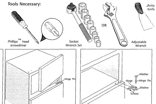
1. Snap off hinge cover at top of cabinet 2. Open the freezer door enough to allow
